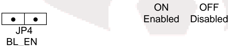
Figure 6: Backlight Enable Option Header – JP4
