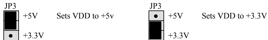
Figure 2: VDD_SEL Option Header
