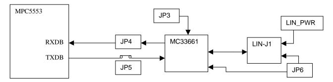
The LIN interface provides optional features of slew rate control, network supply, and wake up option. See the JP3, JP4, JP5, JP6, LIN\_PWR, and CT8 options following.
