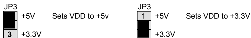
Figure 2: VDD_SEL Option Header – JP3
