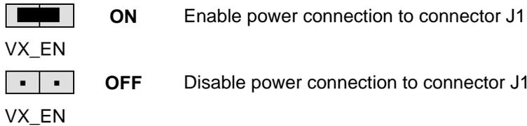
**CAUTION:** Do not apply power to connector J1 while also sourcing power from either the PWR connector or the USB-BDM circuit. Damage to the board may result.
