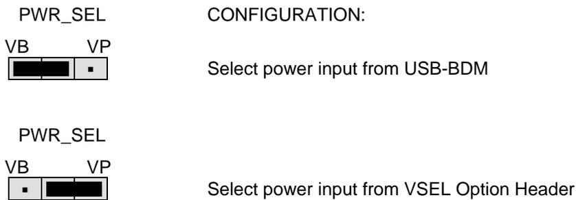
Power from the integrated BDM is drawn from the USB bus and is limited to **500mA**. Excessive current drain will violate the USB specification will cause the USB bus to disconnect.
