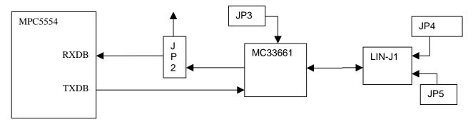
The LIN interface provides optional features of slew rate control, network supply, and wake up option. See the JP2, JP3, JP4, JP5 and CT17 options following.
